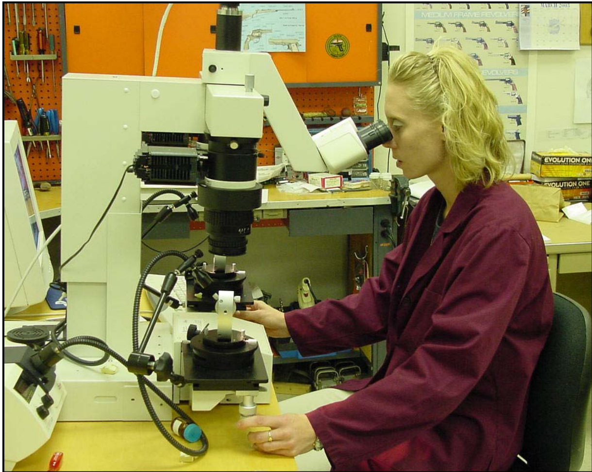
Helen Schumacher, Forensic Lab Criminalist, is using a comparison microscope for the examination of fired bullets and discharged cartridge casings. Helen specializes as a Firearms and Toolmark Examiner.
