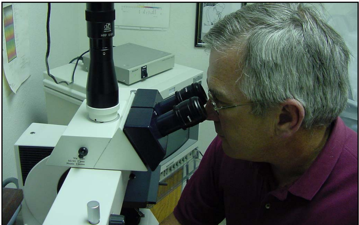
Rex Riis, Director of the Forensic Lab, is using a Comparison P.L.S. Microscope (Polarizing Light Microscope) to examine evidence.
